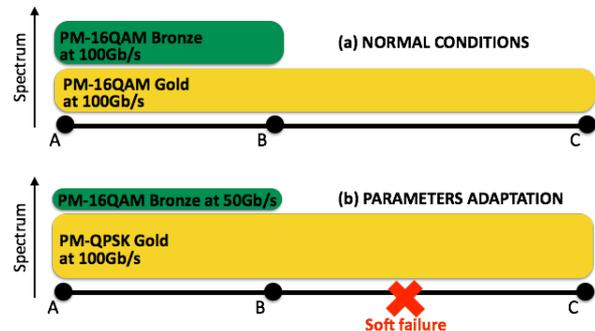
Fig. 1 Example of spectrum sharing before (a) and after (b) a soft failure.
