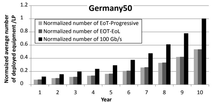
Figure 5: Total normalized number of deployed EOTs and 100 Gb/s interfaces per year, per LP
