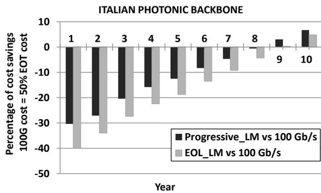
Figure 11. Percentage of cost savings when 100 Gb/s cost = 50% EOT cost and for different cost erosions: EOT (15%), 100 Gb/s (10%)
