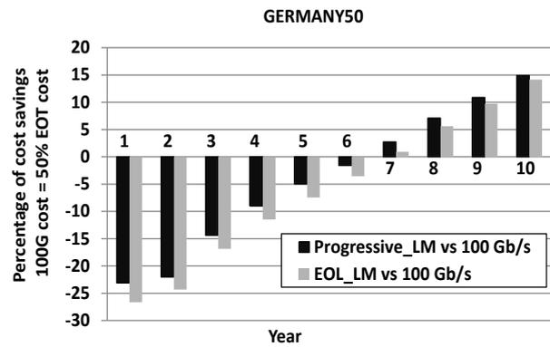
Figure 12. Percentage of cost savings when 100 Gb/s cost = 50% EOT cost and for different cost erosions: EOT (15%), 100 Gb/s (10%)
